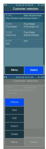
The acquired customer number applies to all subsequent measurements until the device is switched off or another number is selected.
