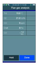
Before starting the measurement, which is displayed in mg/Nm3, mg/MJ, and mg/kWh, you have to select the fuel and the  $O_2$  reference value. The standard  $O_2$  reference value for a fuel is preset.
