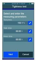
"Next" starts the measurement program. During the measurement, ">>/<<" can be used at any time to switch between table and diagram display.
