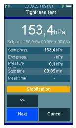
Measurement: The pressure pattern as well as the starting, end and differential pressure are recorded during the measurement period. The selected measurement period can be shortened using "Quit".
