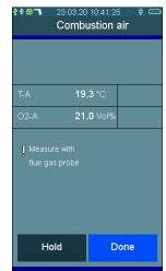
In this case, the combustion air temperature is accepted when determining the measurement readings or during averaging.
