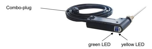
The green LED indicates the exhaust probe being ready for measurement.
