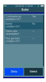
Up to 4 checklists each with a maximum of 20 entries can be created using the PC measurement data management. Each entry can be created so that it can be answered with Yes / No, or with an entry consisting of a max. of 5 characters. If no input has been provided, the entry is shown using ---.
