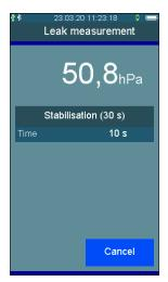
The current pressure, the pressure at the beginning of the measurement, the measurement time elapsed so far, the drop in pressure and the currently calculated leak rate are shown.
