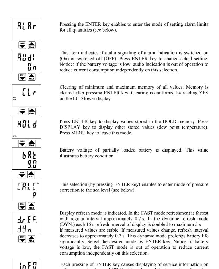
software version (upper LCD line) together with instrument configuration
