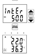
Now instrument displays adjusted storing interval. To modify the storing interval use arrow keys. Interval 10 sec is displayed as **MIN 0:10**, minute intervals are displayed as **MIN x:00** and hour intervals as **x:Ho**. Confirm adjusted interval by pressing ENTER key. Notice: if manual logging mode is selected, this menu item is skipped (there is no interval adjustment).
