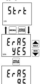
If it is needed to clear the memory before logging start, first it is necessary to select menu item logging START (symbol Strt) and confirm by pressing ENTER kev.
